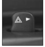
The hazard warning flasher switch is located on the top of the steering column.
